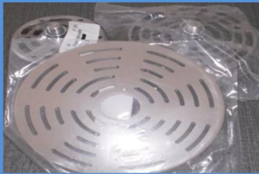
Valve & valve plate High
